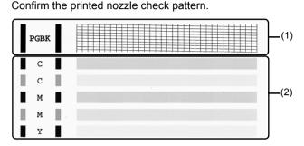
(1) If lines of this pattern are missing, the **Black** print head nozzle needs cleaning. Example: When lines are missing
